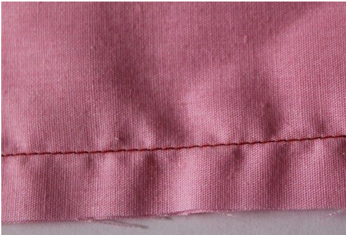
Seam puckering on heavyweight upholstery fabric
